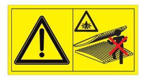
Please consider that a part from the operator who uses the excavator, nobody else is supposed to be in the crushing area of the machine.
