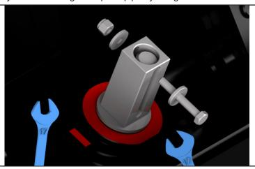
2: unscrew the square pipe by using the 46 wrench. In this way the upper jaw shall descend
