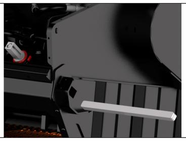
4: screw back into place the loosened square pipe. Make sure that the red perimeter is parallel to the indicator to maintain the correct spring compression.
