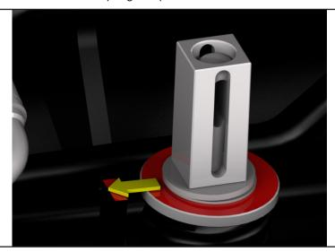
5: reinsert the safety screw making sure that it passes through the threaded bar hole. Check that the shims are tight with the structure and close the compartment by re-tightening the casing screws.
